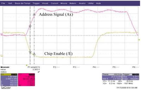
Timing shown from VIL (yellow trace /CS) and VIH (pink for address signal) as delta X = 6ns. Even at actual internal gate switching point (~ VDD/2), the skew is still around 6ns.
