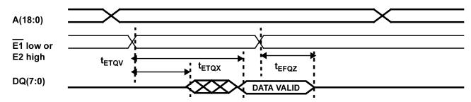
SRAM Read Cycle 2: Chip Enable Access
